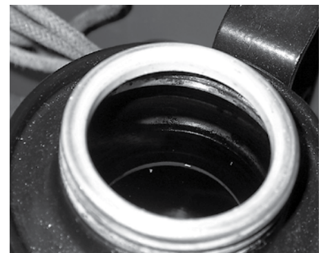
Fluid level has dropped only a few thousandths of an inch and meniscus reflection has disappeared. Compare with photo just above.
